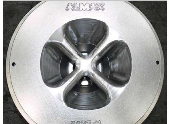
Figure 7. An example of a porthole die designed with dead metal flow control.
