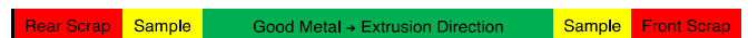
Figure 2. Schematic diagram used to experimentally identify coring and charge weld positions in extrusion.
